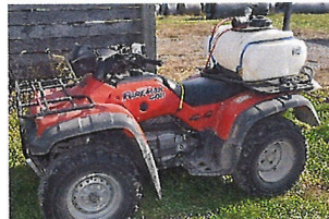
Inexpensive sprayers can be attached to ATVs or golf carts to apply herbicides on small pastures.
